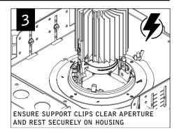
Luminaires must be installed by a qualified electrician (check with local and national codes for proper installation).
