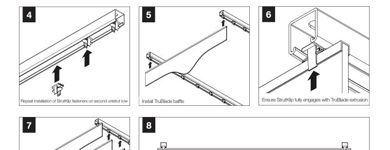
Center and align edges of TruBlade baffles to ensure flush installation
