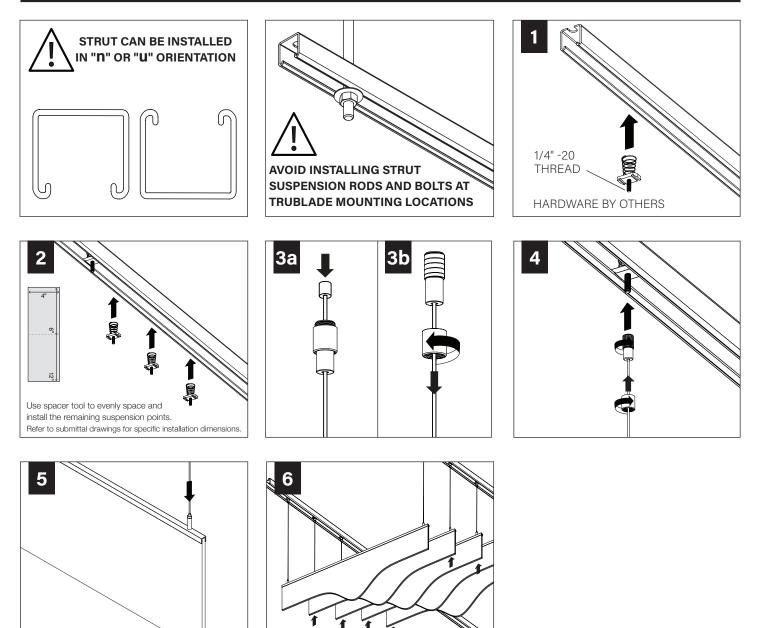
Install remaining TruBlade baffles
