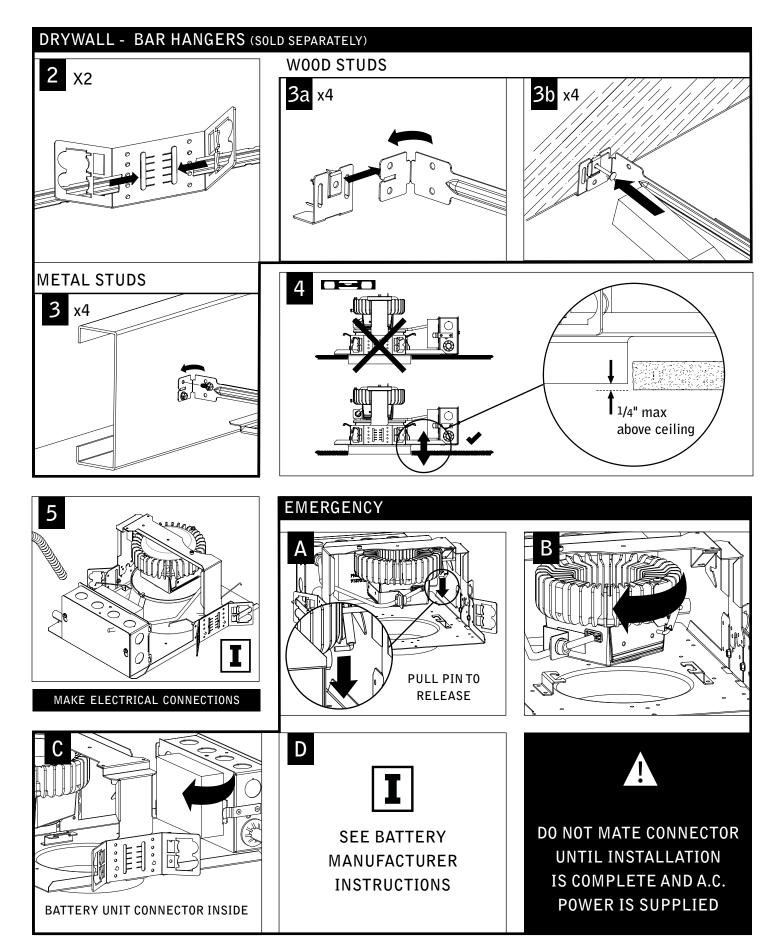
Fixtures must be installed by a qualified electrician (check with local and national codes for proper installation). To prevent electrical shock, disconnect electrical supply before installation or servicing.
