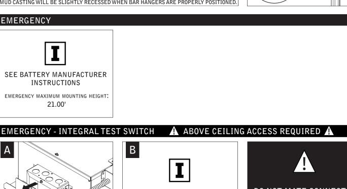
**DO NOT MATE CONNECTOR** UNTIL INSTALLATION IS COMPLETE AND A.C. **POWER IS SUPPLIED**
