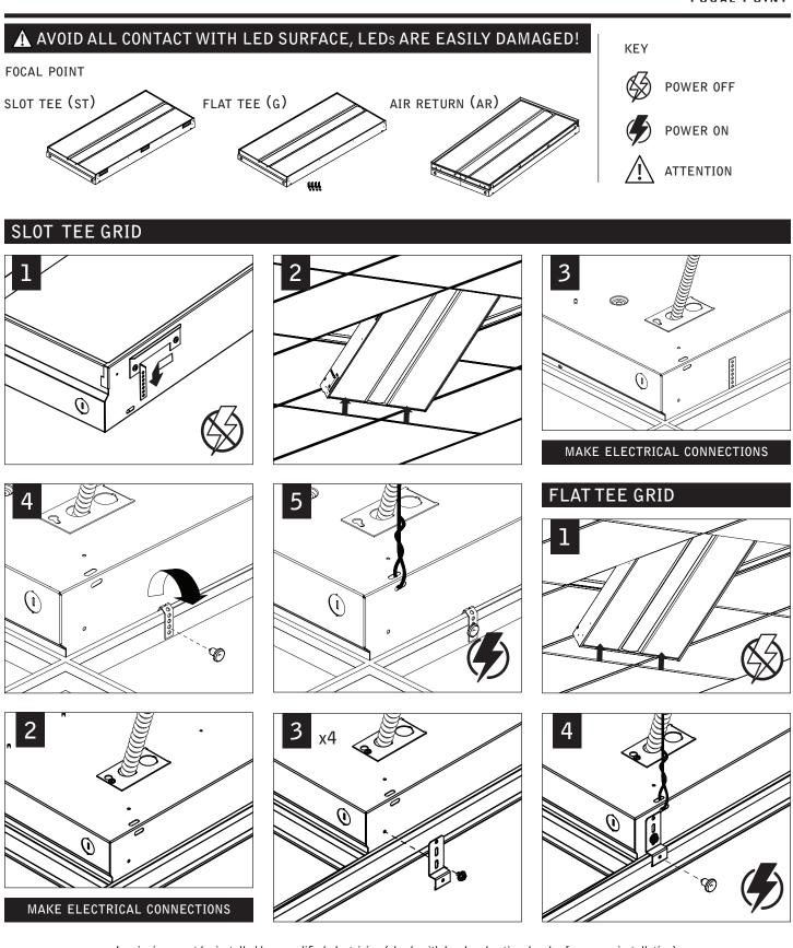
Luminaires must be installed by a qualified electrician (check with local and national codes for proper installation). To prevent electrical shock, disconnect electrical supply before installation or servicing.
