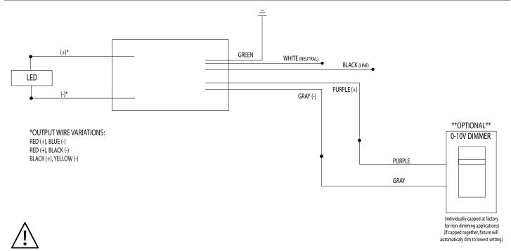
REFERENCE DRIVER MANUFACTURER'S SPEC SHEETS FOR DRIVER SPECIFIC WIRING DIAGRAMS. EMERGENCY LUMINAIRES WIRED ACCORDING TO BATTERY MANUFACTURER'S INSTRUCTIONS.
