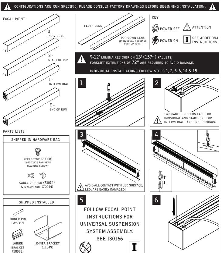
Luminaires must be installed by a qualified electrician (check with local and national codes for proper installation). To prevent electrical shock, disconnect electrical supply before installation or servicing.
