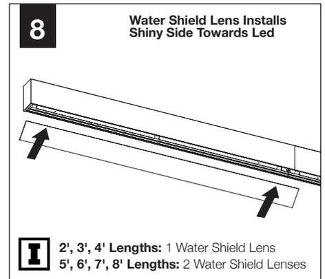
**Water Shield Lens Installs
