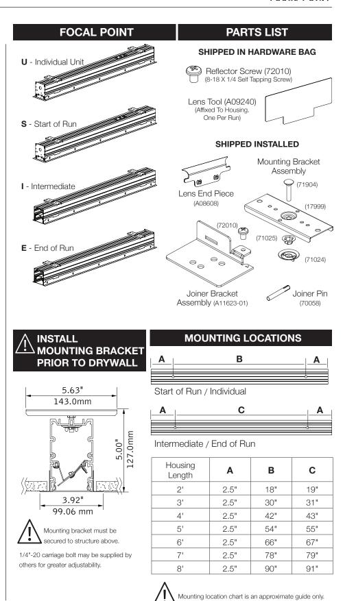
**NEW CONSTRUCTION ONLY** Configurations are run specific, please consult factory drawings before beginning installation.
