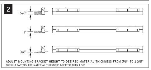
SECURE MOUNTING BRACKET TO INSTALLATION SUPPORTS, IF APPLICABLE (HARDWARE BY OTHERS)
