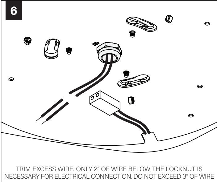
TRIM EXCESS WIRE. ONLY 2" OF WIRE BELOW THE LOCKNUT IS
