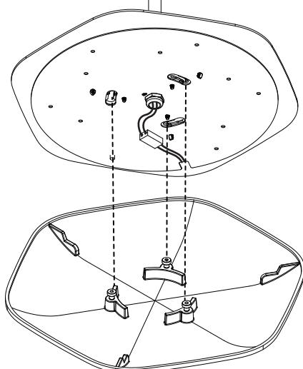
ALIGN PEGS ON FACE PLATE TO SLOTS ON LED MODULE.
