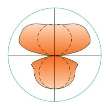
Batwing indirect distribution is achieved delivering superior ceiling uniformity and shadow-free illumination above the void.
