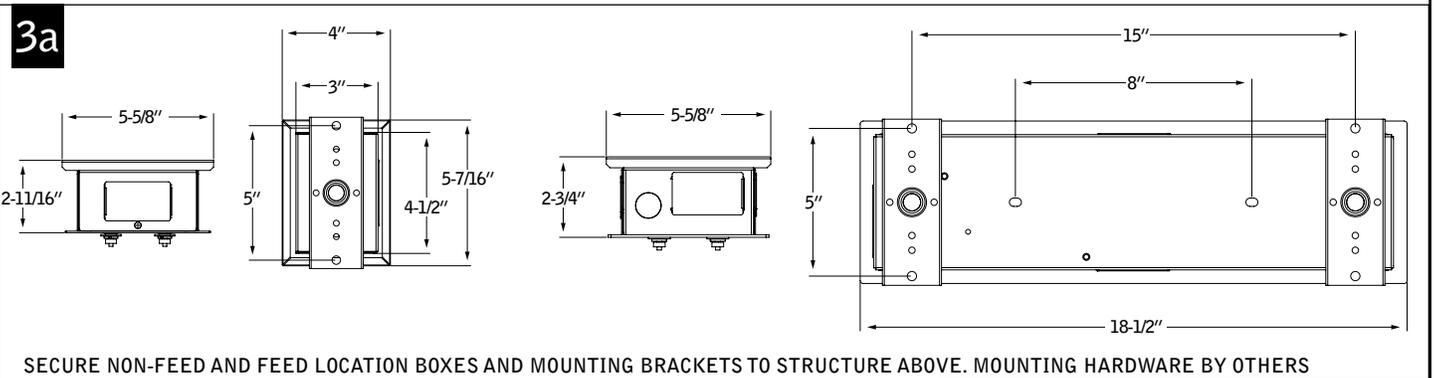
SECURE NON-FEED AND FEED LOCATION BOXES AND MOUNTING BRACKETS TO STRUCTURE ABOVE. MOUNTING HARDWARE BY OTHERS
