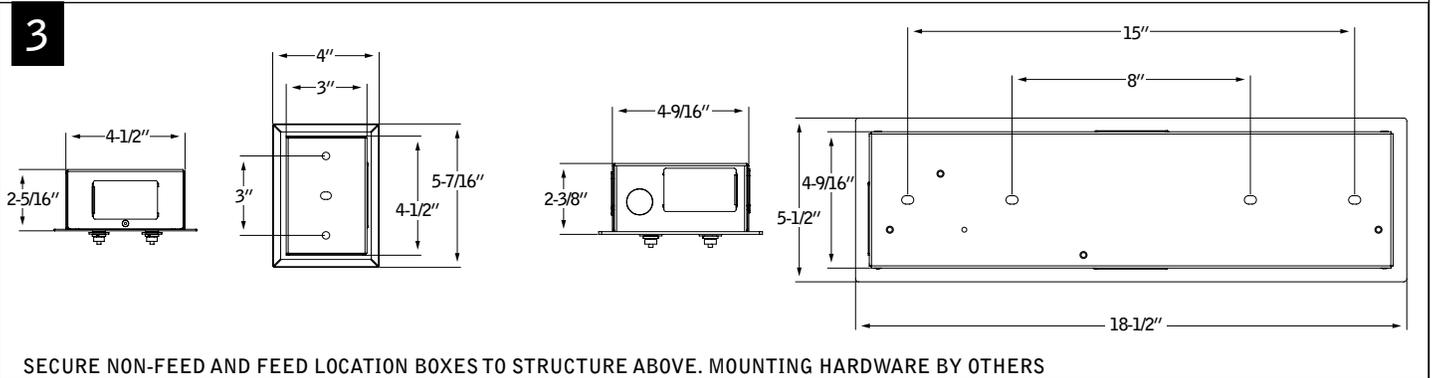
SECURE NON-FEED AND FEED LOCATION BOXES TO STRUCTURE ABOVE. MOUNTING HARDWARE BY OTHERS
