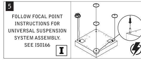
Luminaires must be installed by a qualified electrician (check with local and national codes for proper installation). To prevent electrical shock, disconnect electrical supply before installation or servicing.
