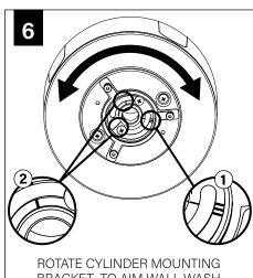
BRACKET TO AIM WALL WASH MARKING TOWARDS WALL
