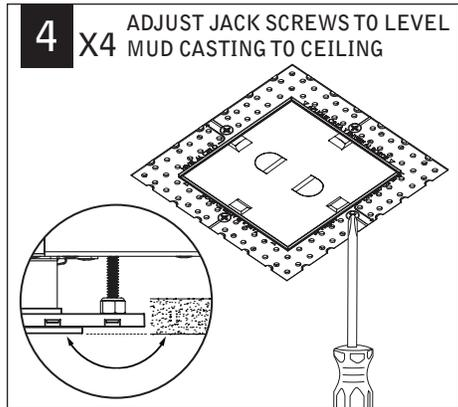
MUD CASTING WILL BE SLIGHTLY RECESSED WHEN BAR HANGERS ARE PROPERLY POSITIONED.
