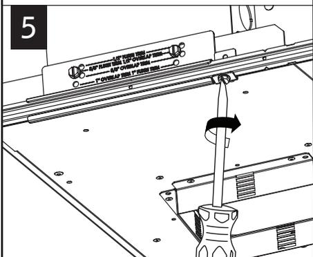
TIGHTEN SCREW TO SECURE BAR HANGER IN PLACE
