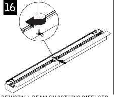
REINSTALL BEAM SMOOTHING DIFFUSER
