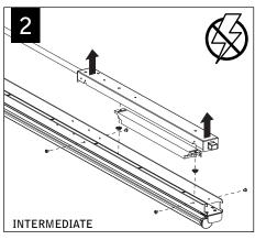
Luminaires must be installed by a qualified electrician (check with local and national codes for proper installation). To prevent electrical shock, disconnect electrical supply before installation or servicing.
