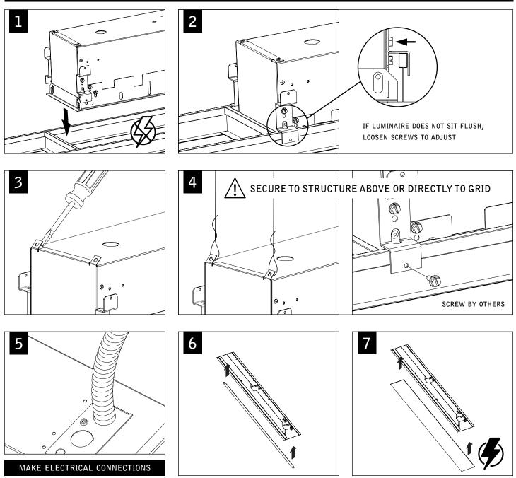
Luminaires must be installed by a qualified electrician (check with local and national codes for proper installation). To prevent electrical shock, disconnect electrical supply before installation or servicing.
