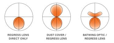
A regressed lens and larger aperture soften the incident luminance and glare, meeting the requirements of the WELL Building Standard™ of 6,000 cd/m2 or less between 45° and 90° from nadir. Refer to WELL v2 Feature L04 on the WELL website for more details.
