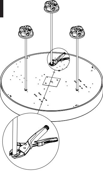
1. ATTACH THE STEM TO COVER. DO NOT OVER TIGHTEN STEM, THIS MAY CAUSE PINCHED WIRES.
