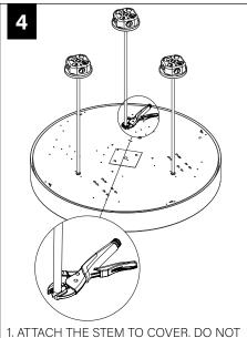
OVER TIGHTEN STEM, THIS MAY CAUSE PINCHED WIRES.
