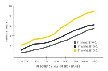
Sabins per unit is a measure of the amount of sound absorption in one baffle. Absorption per unit and total absorption will vary based on the configuration of each array. Consult the ASTM C423 reports for more information.
