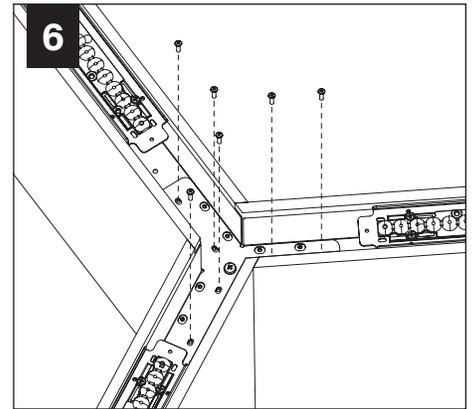
**⚠ DO NOT PINCH WIRES BENEATH PLATE.**
