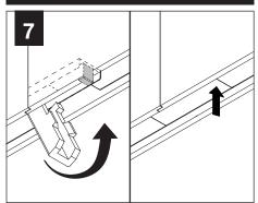
GENTLY FLIP UP PET FELT ACCESS DOOR UNTIL IT MEETS THE INTERNAL STOPPING MECHANISM
