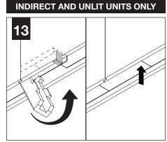
GENTLY FLIP UP PET FELT ACCESS DOOR UNTIL IT MEETS THE INTERNAL STOPPING MECHANISM
