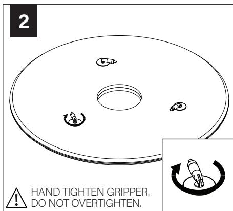
! HAND TIGHTEN GRIPPER.
