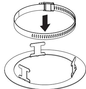
INSTALL CLAMP ONTO THE OUTSIDE OF THE TABS ON THE CANOPY CAPTURE (DO NOT TIGHTEN)
