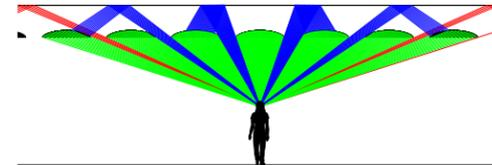
98% of the sound is captured either directly in the shade, or indirectly after reflecting off the ceiling to the back of the domed shade.
