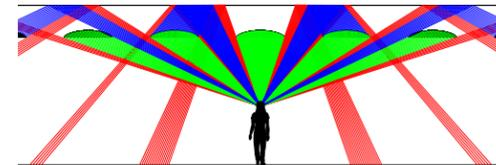
83% of the sound is captured either directly in the shade, or indirectly after reflecting off the ceiling to the back of the domed shade.
