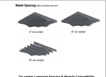
**On-center Luminaire Spacing & Module Compatibility** Use the table below to determine suitable module sizes based on the desired on-center spacing of the luminaires.
