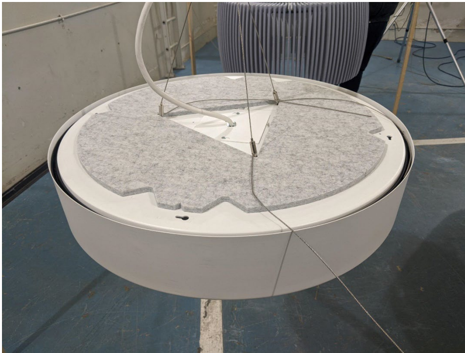
Figure 3 – Individual specimen light unit prior to installation of felt fins around perimeter
