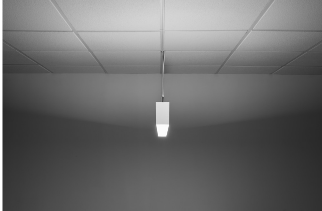
The broad distribution of the Indirect batwing optic allows for spacing up to 16' on center with 3:1 ceiling uniformity with a 24" suspension.
