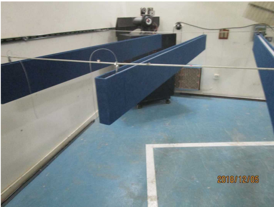
Figure 2 - Detail of individual baffles
