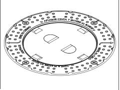
MUD CASTING WILL BE SLIGHTLY RECESSED WHEN BAR HANGERS ARE PROPERLY POSITIONED.
