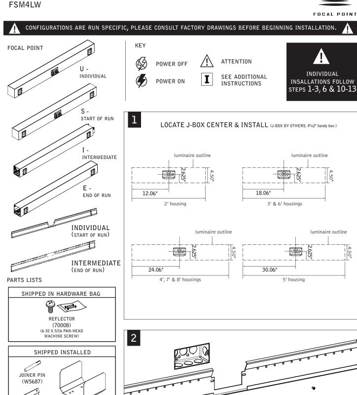
Luminaires must be installed by a qualified electrician (check with local and national codes for proper installation).
