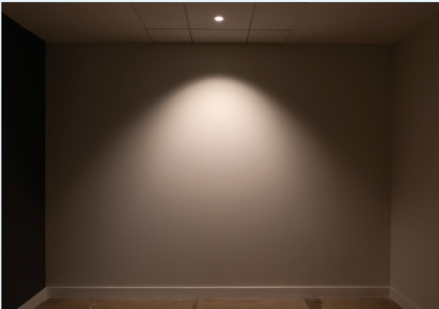
60° wide flood (WFL) clear diffuse reflector (CD) center beam candlepower: 1275
