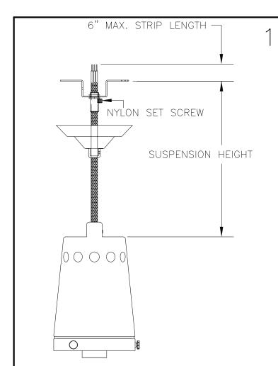
DETERMINE DESIRED SUSPENSION LENGTH. CUT CORD WITH 6" EXCESS (EX. 3' DESIRED SUSPENSION=3'-6" CORD LENGTH). ADJUST J-BOX BRACKET ALONG CORD UNTIL TOP OF BRACKET IS AT DESIRED CEILING SUSPENSION POINT. TIGHTEN BRACKET ONTO CORD WITH NYLON SET SCREW. STRIP CORD ABOVE J-BOX BRACKET WITH IDEAL #45-128 OR EQUAL COAX STRIPPER.
