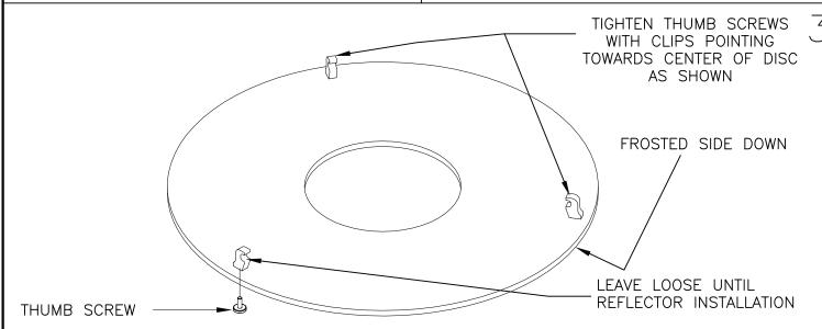
INSTALLATION OF OPTIONAL ACRYLIC DIFFUSER to be completed before installation of reflector onto housing. Insert thumb screws through holes on frosted side of diffuser and screw into clips. Adjust clips as shown by tightening 2 of 3 thumb screws with clips pointing toward the center of the disc. Slide curled edge of reflector into 2 tightened clips. Turn and tighten 3rd clip down.
