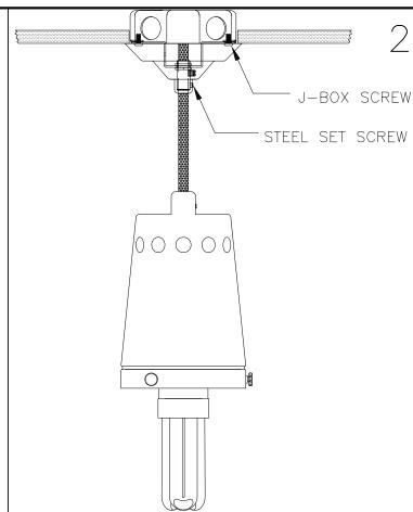
ATTACH J-BOX BRACKET TO J-BOX WITH J-BOX SCREWS (BY OTHERS). MAKE POWER CONNECTIONS. SLIDE CANOPY UP UNTIL FLUSH WITH CEILING, TIGHTEN CANOPY SET SCREW AGAINST BRASS COUPLER (DO NOT OVER TIGHTEN SET SCREW). 1 LAMP FIXTURES: AFTER HOUSING IS SECURE, INSTALL LAMP. 2 LAMP FIXTURES: INSTALL LAMPS AFTER STEP 4 IS COMPLETE. TO INSTALL LAMP: INSERT LAMP INTO SOCKET AND TWIST CLOCKWISE TO LOCK.
